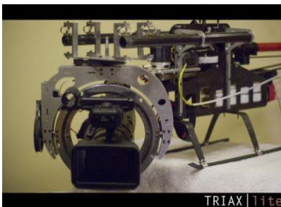
1 st Generation: TRIAX|lite Installation
